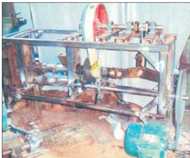
Newly designed mini seed oil expeller for Pongamia and Jatropha
