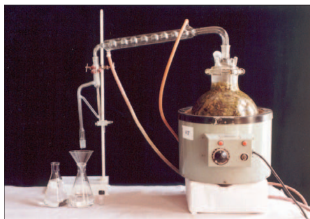
Modified extraction assembly
