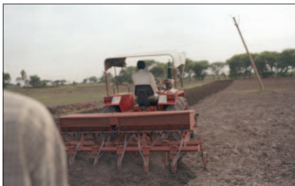
CRIDA planter for timely sowing of maize in Vertisols
