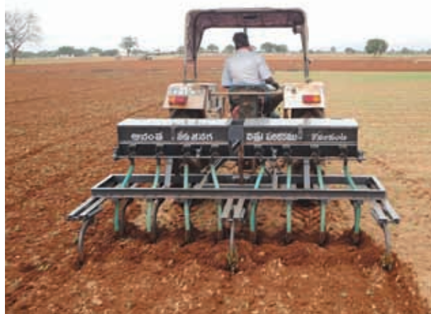
Sowing of groundnut using tractor drawn Ananta planter (left) and field view of groundnut (right)
