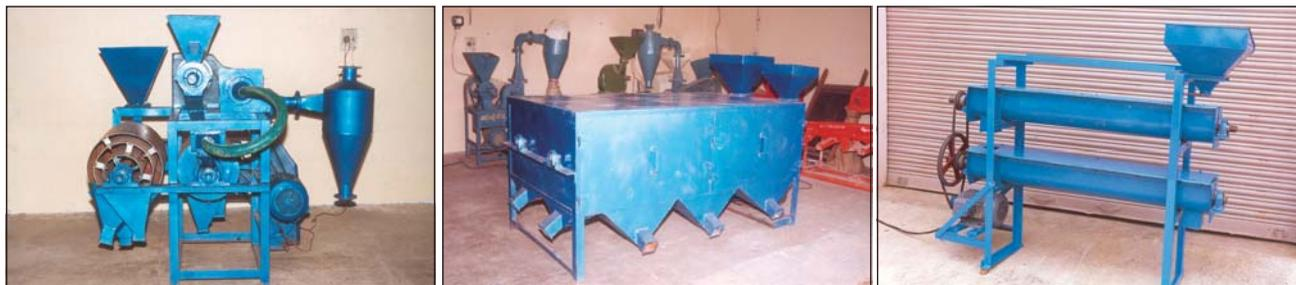
Modified IIPR dalmill (left), rotary screen grader (center) and polishing machine (right)
