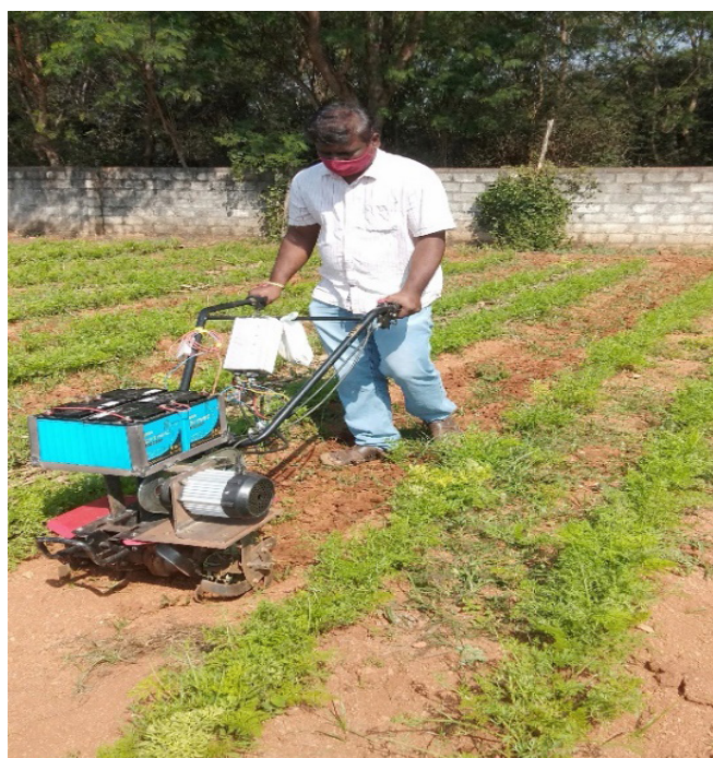
Solar-cum-battery operated weeder in operation
