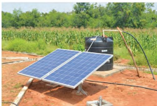
A small scale solar powered micro-irrigation system was designed and installed for the demonstration and use of small farmers having  $\leq 1$  acre land under IFS module for growing vegetables under farm pond system.
