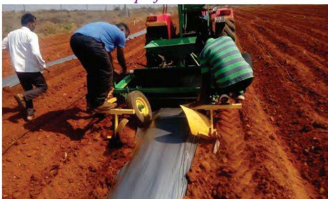
*Mulching sheet laying machine demonstration in farmer fieldcrop*
