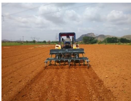
Sowing of groundnut with tractor drawn Anantha groundnut planter
