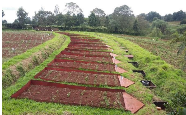
Fig 2. Runoff plots installed at right angle to the contours and parallel to the slope
