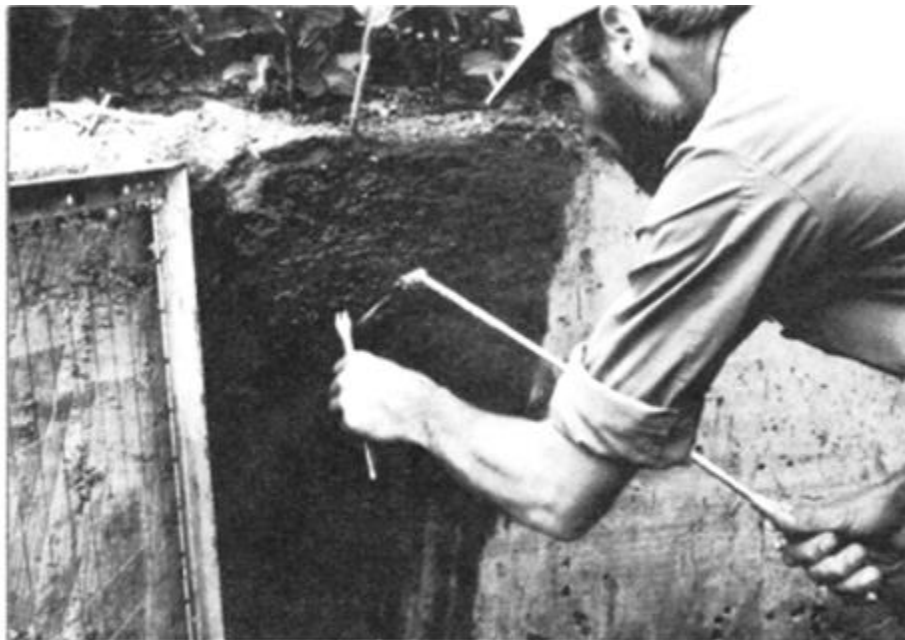
Fig. A thin layer of soil is washed and scraped from the prepared face of an Ida silt loam soil profile. A square grid (left) is then placed on the soil face to allow root location and numbers to be determined in the trench profile method.
